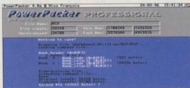
You can increase the storage capacity of your hard drive or floppy disks by compressing the files with PowerPacker professional
